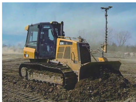
The Cat D5K2 with Topcon system during the GPS class at Lynnville.
